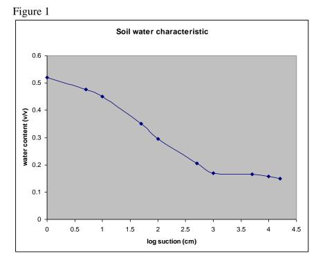
Figure 1 is an example of a typical soil water characteristic. Field capacity, for the example here corresponds to a log suction of 2, i.e. a water content of 0.3. The drier end of the characteristic is controlled by the soil texture while at the wetter end the soil structure dominates the relationship.
